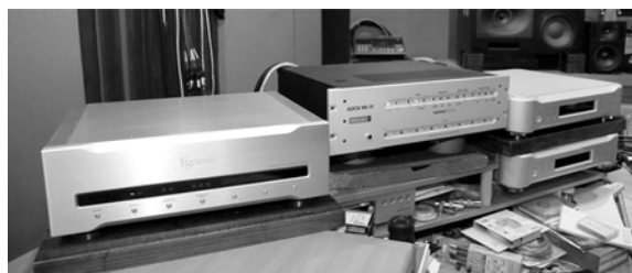
Rubidium master clock generator G-0Rb (left). A set of D/A mono-block converters D-01 (right).
